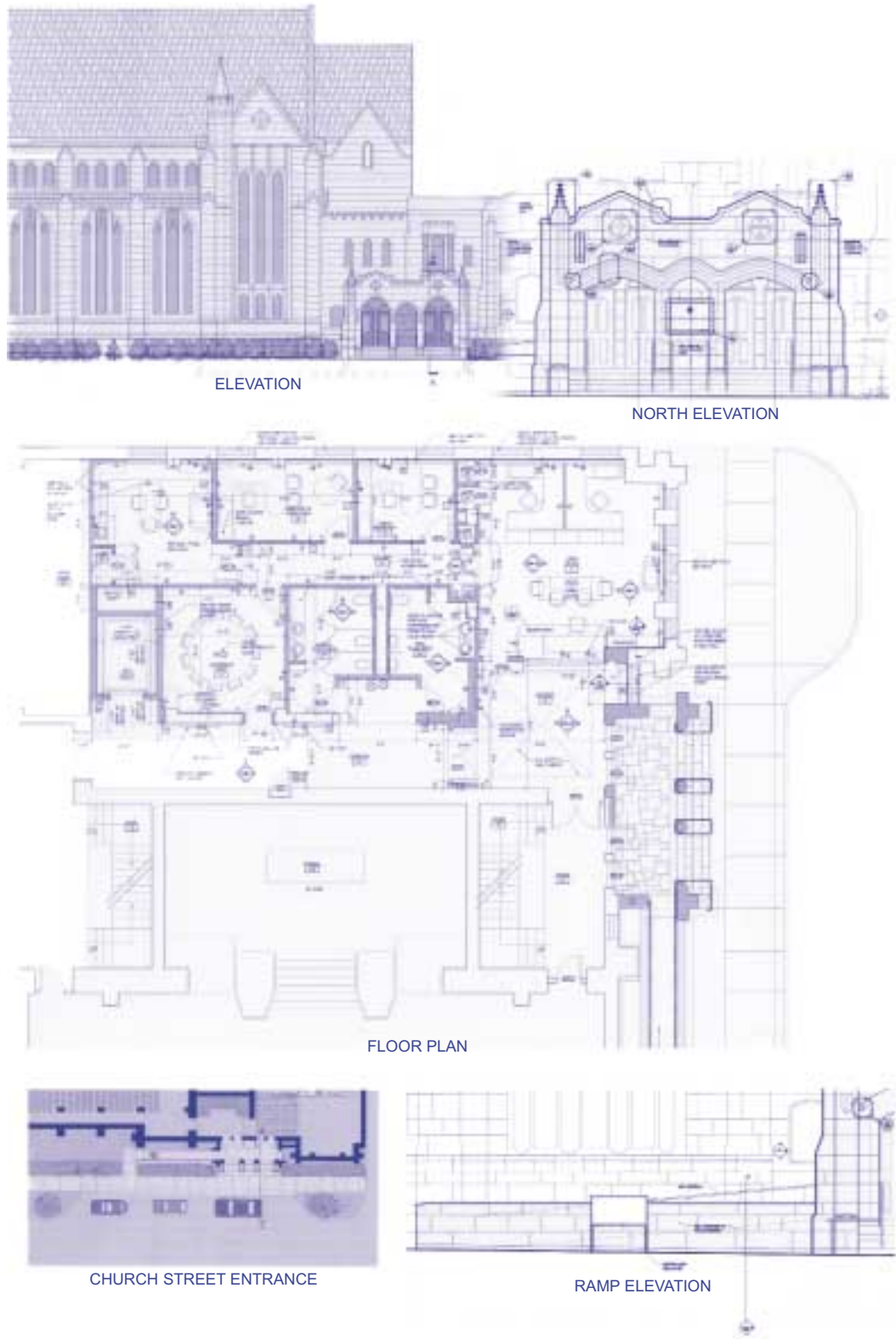
Figure 17: These working drawings detail accessibility alterations to be made to an existing church. The improvements take design cues from the original building. Courtesy of Yas/Fischel Architects
